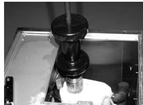
Using Slide Hammer
