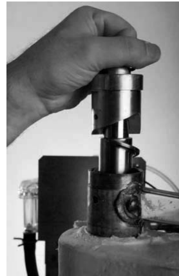
Pull Auger Up and Out
