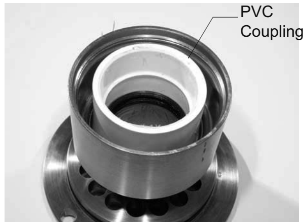
Inserting Lip Seal Using PVC Coupling
