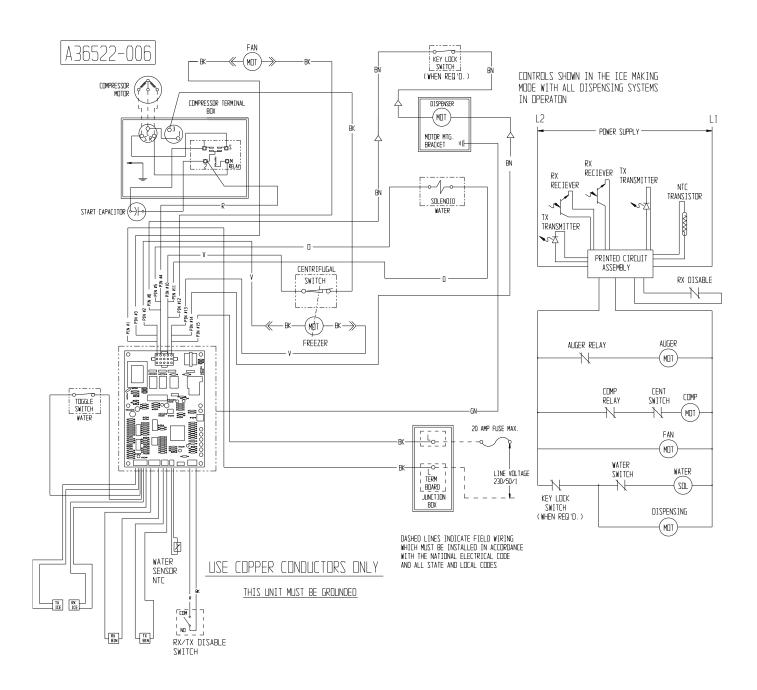
MDT3 or MDT4 Wiring Diagram with Contactor (change in early 2011)
