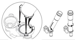
**INSTALL O-RING** onto discharge tube. Apply food equipment lubricant on o-ring.
