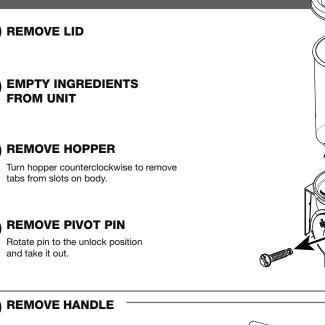
Lift handle upward to the position just before it would click. This makes the handle easier to remove.
