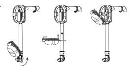
Press dome into housing fully.
