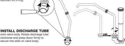
onto valve body. Rotate discharge tube clockwise and press down firmly to secure into slots on valve body.
