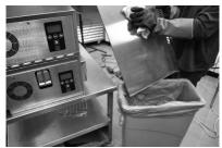
Spray a clean, sanitizer-soaked towel with Heavy Duty De-greaser solution then wipe down the in-feed rack. Rinse the in-feed rack with a separate, clean sanitizer soaked towel.
