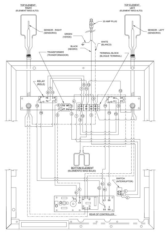
FOR REFERENCE WIRING DIAGRAM IS SHOWN AS UNIT IS ASSEMBLED WITH THE BOTTOM PLATE REMOVED. THE TOP DESCRIPTIONS ARE THEIR POSITIONS WHEN UPRIGHT.
