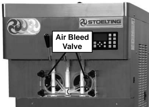
Figure 3-8 Air Bleed Valve
