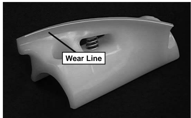
Figure 3-3 Auger Flight Wear
