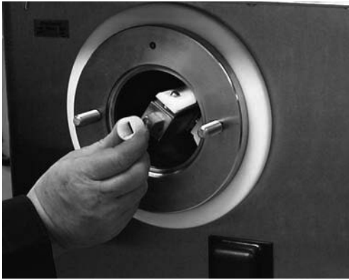
Figure 3-7 Install Front Wear Bushing
