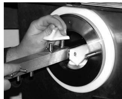
Figure 3-6 Installing Auger Blades
