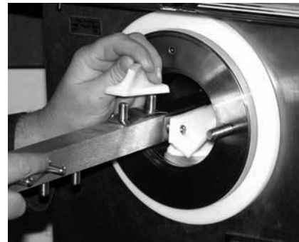
Figure 3-6 Installing Auger Blades
