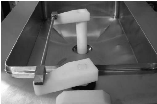
Figure 3-3 Flow Control Assembly
