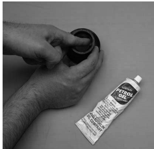
Figure 3-5 Lubricate Rear Seal
