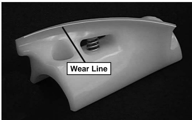
Figure 3-3 Auger Flight Wear
