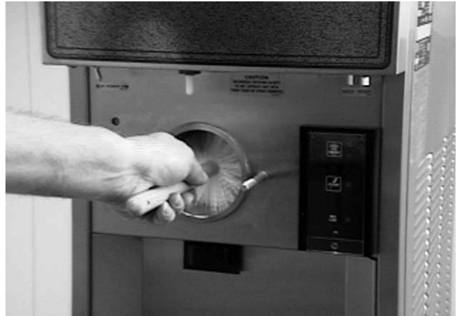
Figure 24. Cleaning Freezer Barrel
