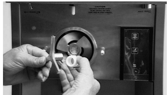
Figure 21. Removing Auger Support
