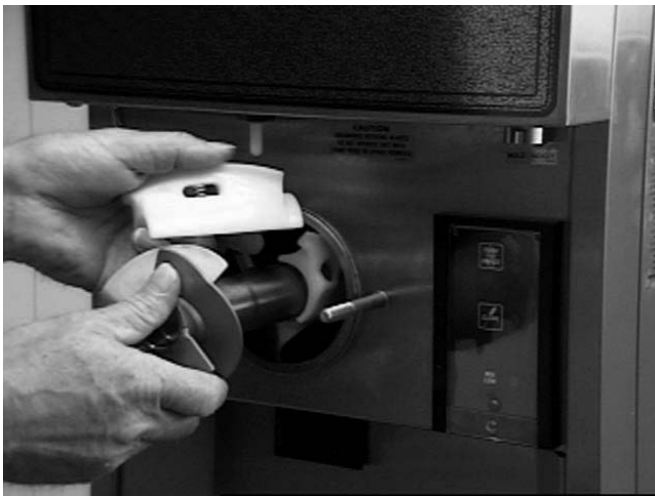
Figure 22. Auger Shaft Removal
