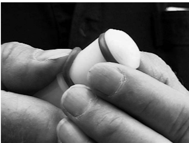
Figure 23. Removing "O" Ring
