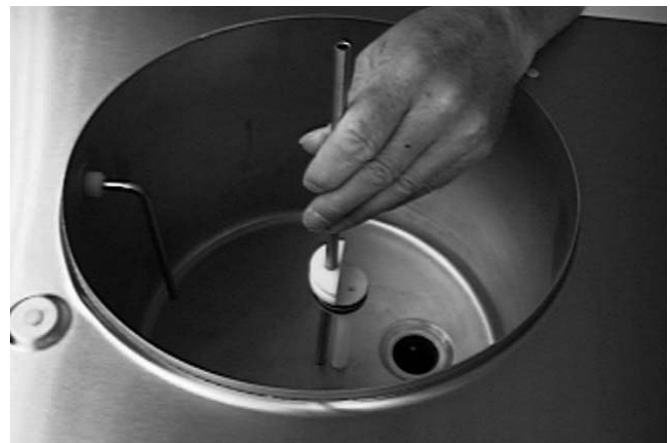
Figure 16. Removing Mix Inlet Regulator
