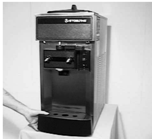
Figure 7. Installing Tray and Cover
