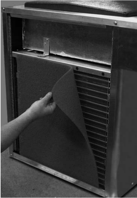
Figure 3-8 F112 Condenser Filter Removal
