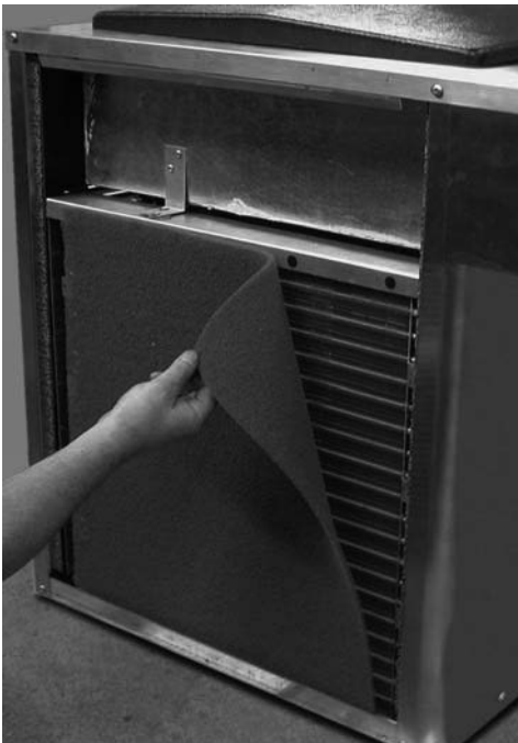
Figure 4-4 F112 Condenser Filter Removal
