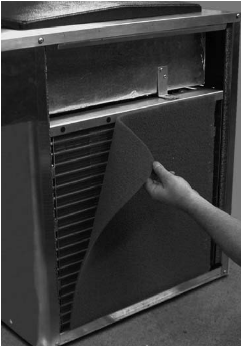
Figure 3-8 F122 Condenser Filter Removal
