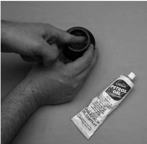
Figure 3-6 Lubricate Rear Seal
