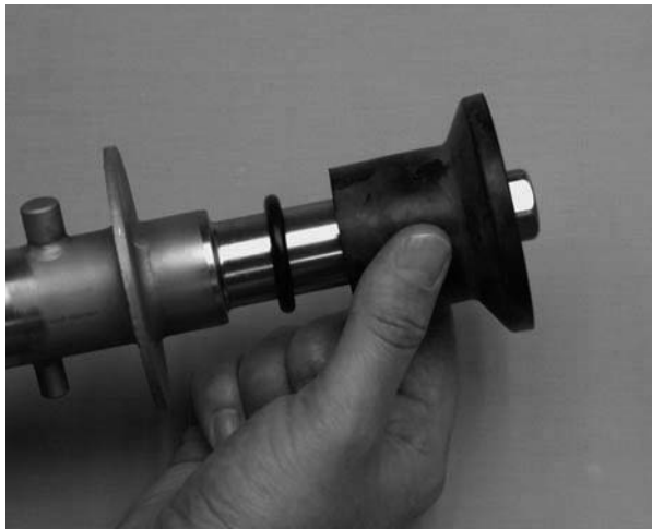
Figure 3-5 Rear Seal Assembly
