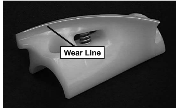
Figure 3-3 Auger Flight Wear
