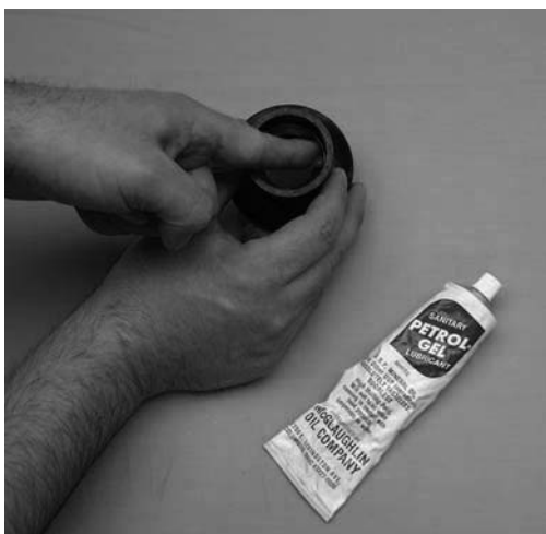
Figure 3-6 Lubricate Rear Seal
