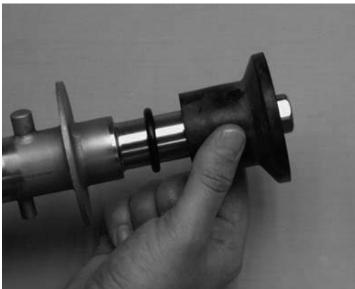
Figure 3-5 Rear Seal Assembly
