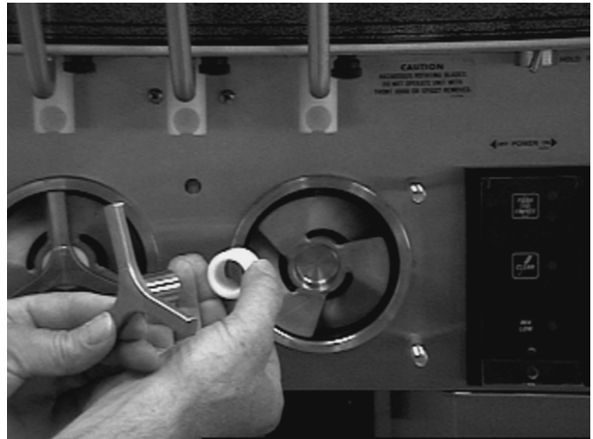
Figure 21. Removing Auger Supports
