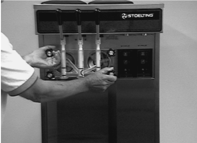
Figure 19. Removing Front Door
