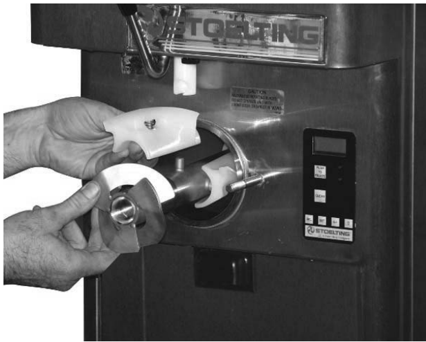
Figure 3-5 Removing Auger Shaft and Flights
