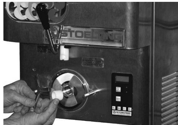
Figure 3-4 Removing Auger Support
