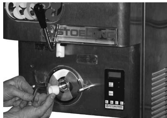
Figure 3-4 Removing Auger Support
