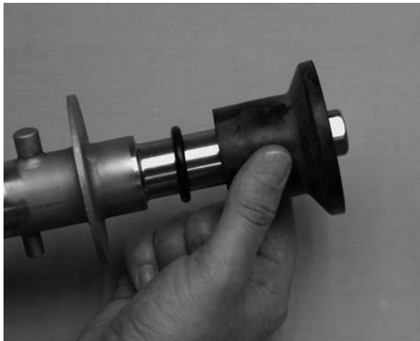
Figure 3-5 Rear Seal Assembly
