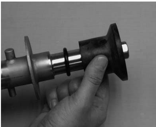
Figure 3-5 Rear Seal Assembly
