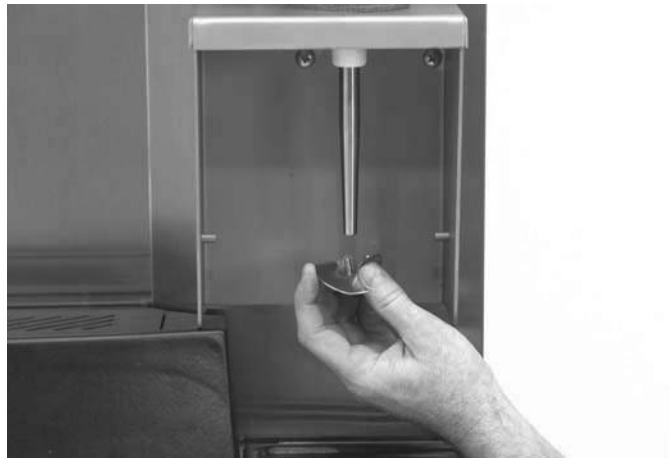
Figure 22. Removing Agitator From Shaft
