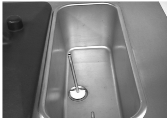
Figure 27. Install Mix Inlet Regulators
