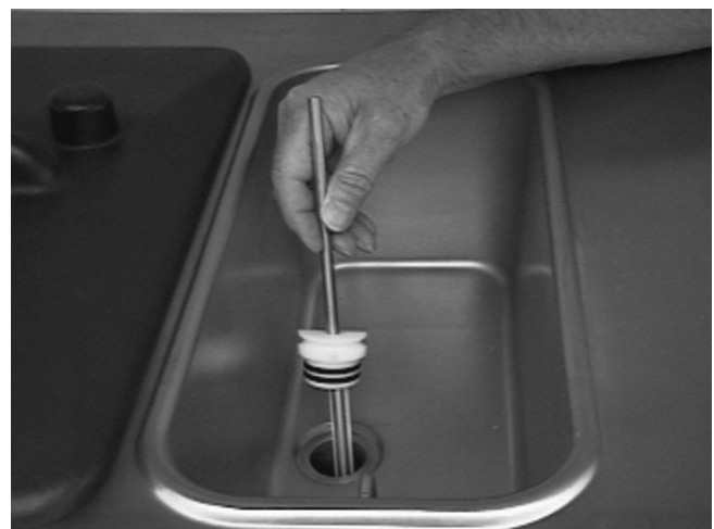
Figure 16. Removing Mix Inlet Regulator
