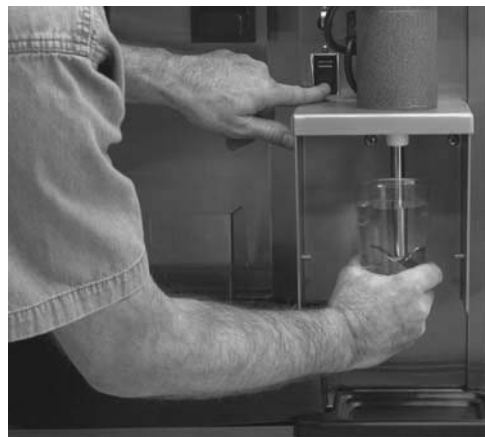
Figure 18. Cleaning Agitator Shaft
