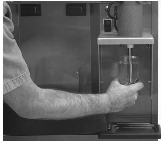
Figure 14. Sanitizing Agitator Shaft (SF144 Model Only)
