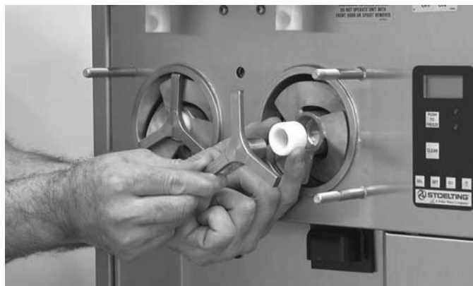
Figure 23. Removing Auger Supports
