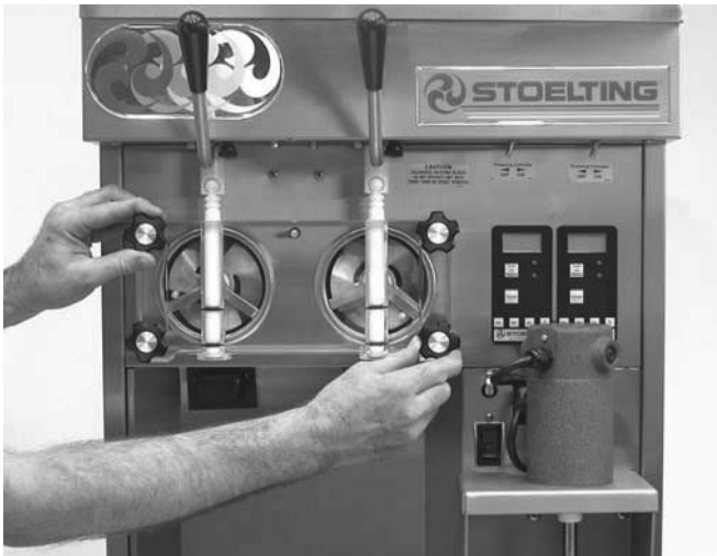
Figure 20. Removing Front Door
