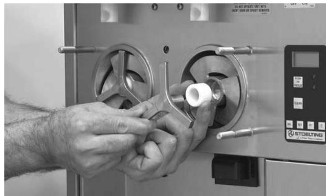
Figure 23. Removing Auger Supports
