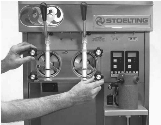
Figure 20. Removing Front Door
