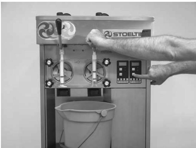
Figure 13. Spigot Opened and Solution Draining
