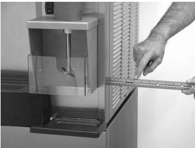
Fig. 4. Space and Ventilation Requirements
