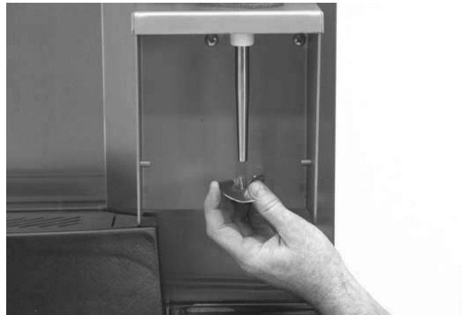
Figure 22. Removing Agitator From Shaft
