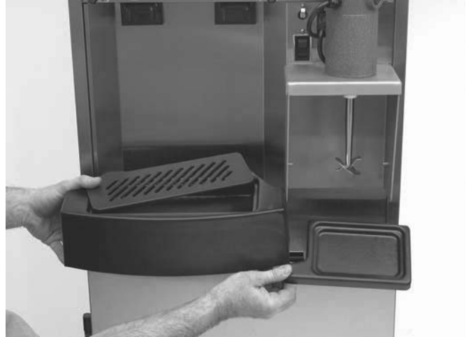
Figure 5. Installing Trays and Inserts (SF144 shown)
