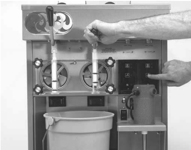
Figure 14. Spigot Opened and Solution Draining
