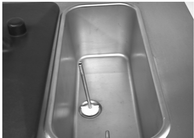
Figure 28. Install Mix Inlet Regulators
