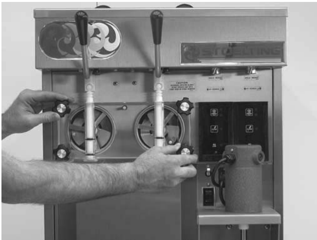
Figure 21. Removing Front Door
