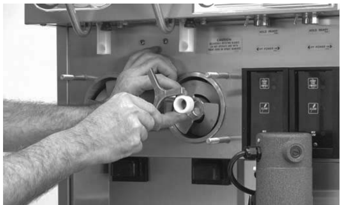
Figure 24. Removing Auger Supports
