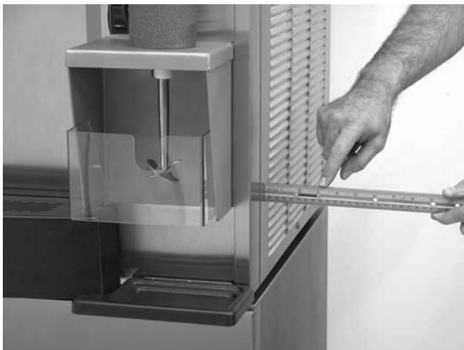
Fig. 4. Space and Ventilation Requirements
