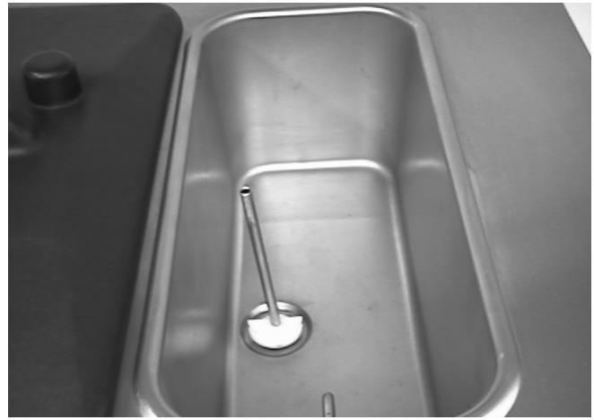
Figure 10. Mix Inlet Regulator
