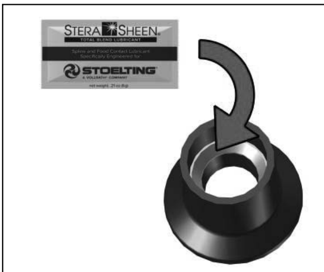
Figure 3-6 Lubricate Rear Seal
