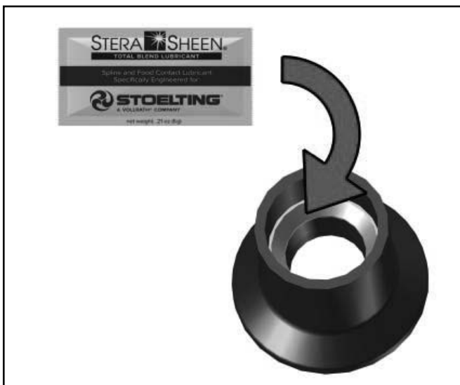
Figure 3-6 Lubricate Rear Seal
