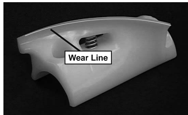
Figure 3-3 Auger Flight Wear
