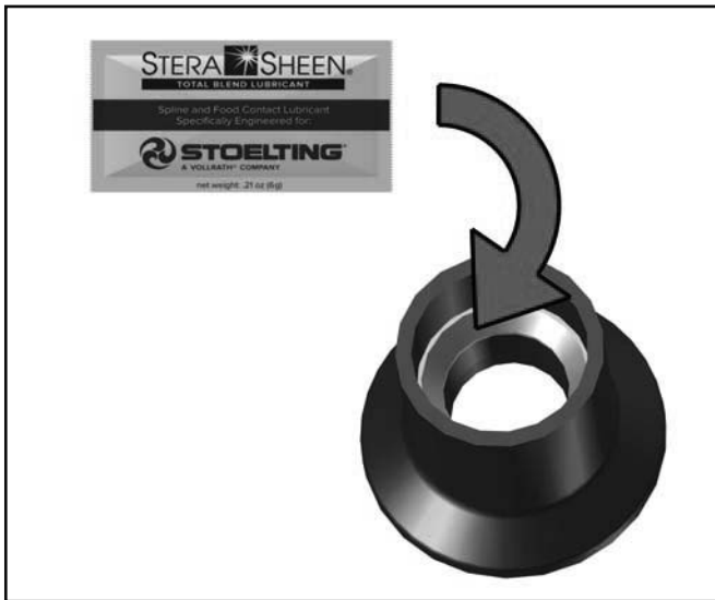
Figure 3-6 Lubricate Rear Seal
