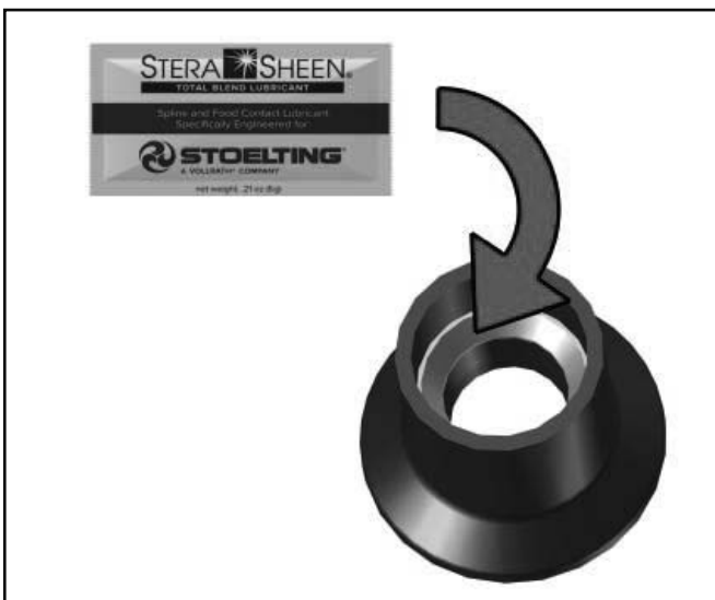
Figure 3-6 Lubricate Rear Seal
