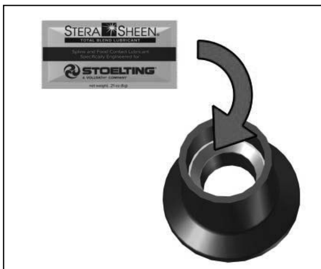
Figure 3-6 Lubricate Rear Seal
