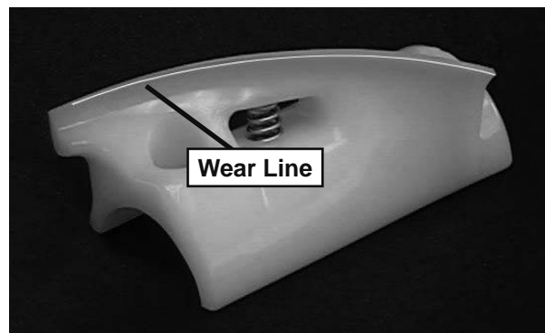
Figure 3-3 Auger Flight Wear
