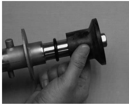
Figure 3-5 Rear Seal Assembly
