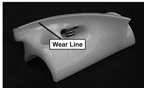
Figure 3-3 Auger Flight Wear
