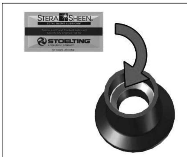
Figure 3-6 Lubricate Rear Seal
