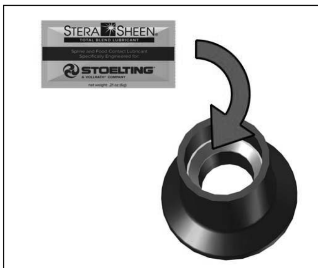
Figure 3-6 Lubricate Rear Seal
