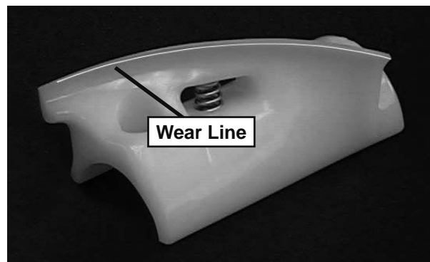
Figure 3-3 Auger Flight Wear
