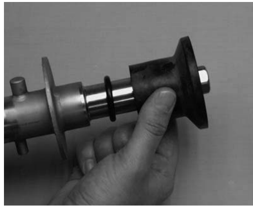
Figure 3-5 Rear Seal Assembly
