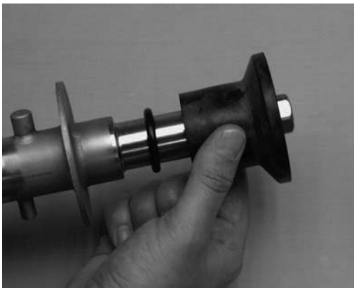
Figure 3-5 Rear Seal Assembly
