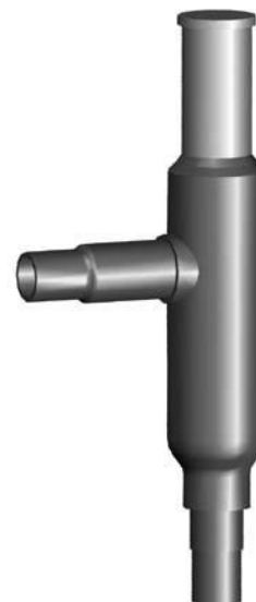
Figure 5-8 Hot Gas Bypass
