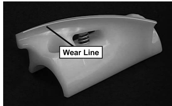
Figure 3-3 Auger Flight Wear
