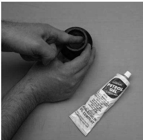
Figure 3-6 Lubricate Rear Seal
