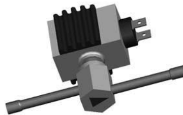
Figure 5-11 Liquid Line Solenoid Valve
