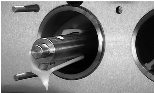
Figure 3-5 Auger Flight Removal
