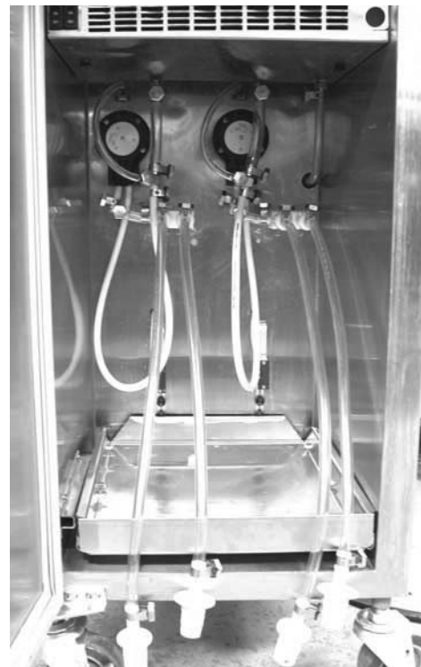
Figure 2-7 Completed BCS Hose Assembly
