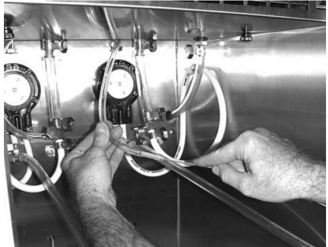
Figure 3-18 Cleaning Air Tube
