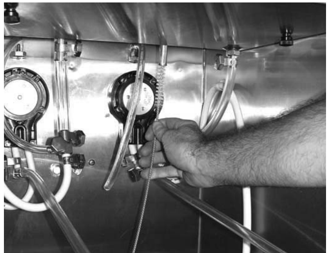
Figure 3-19 Cleaning Feed Tube
