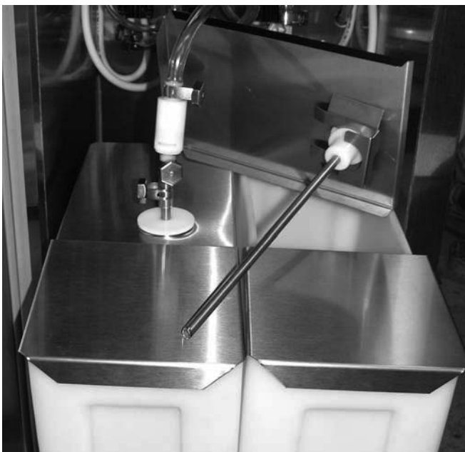
Figure 2-5 Connecting Mix Pick-up Assembly
