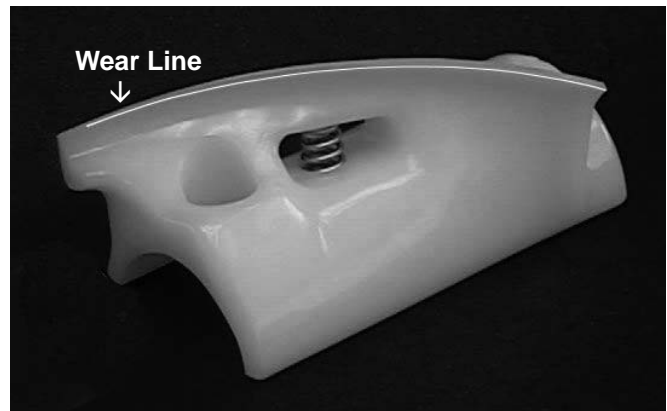
Figure 3-3 Auger Flight Wear
