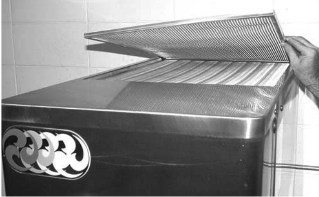
Figure 4-4 Removing Condenser Filter
