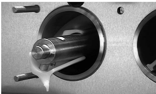
Figure 3-5 Auger Flight Removal
