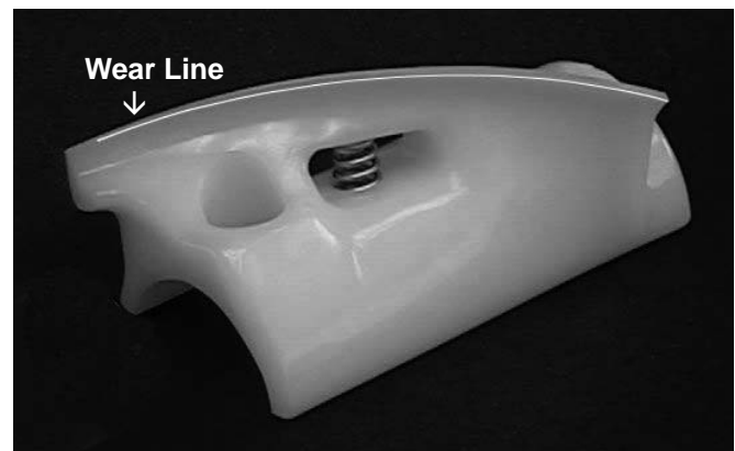
Figure 3-3 Auger Flight Wear
