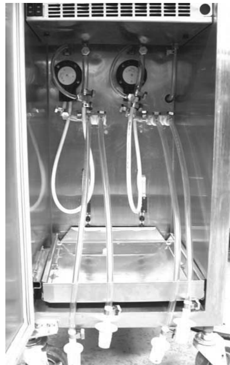
Figure 2-7 Completed BCS Hose Assembly
