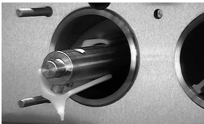
Figure 3-5 Auger Flight Removal
