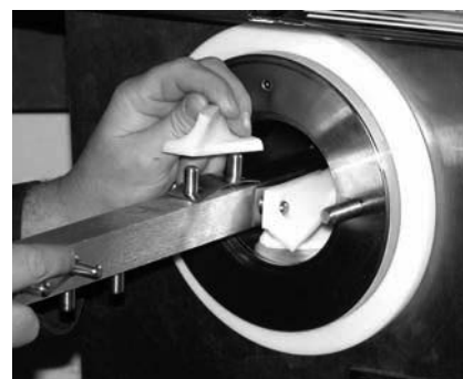
Figure 3-6 Installing Auger Blades
