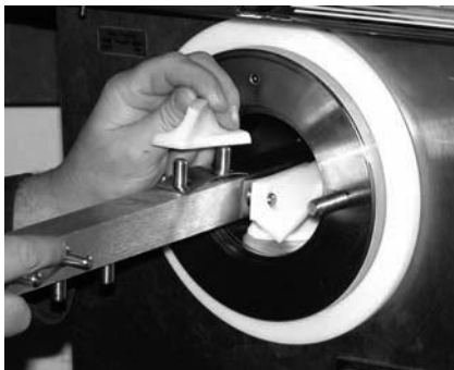
Figure 3-5 Installing Auger Blades
