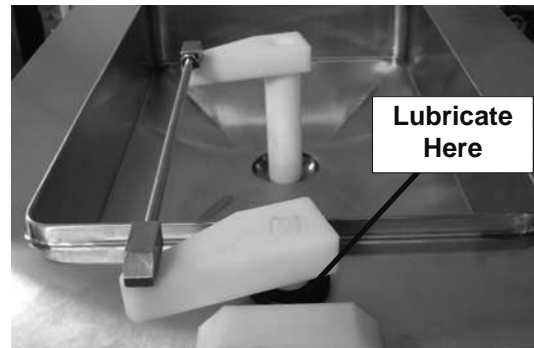
Figure 3-6 Flow Control Arm Lubrication
