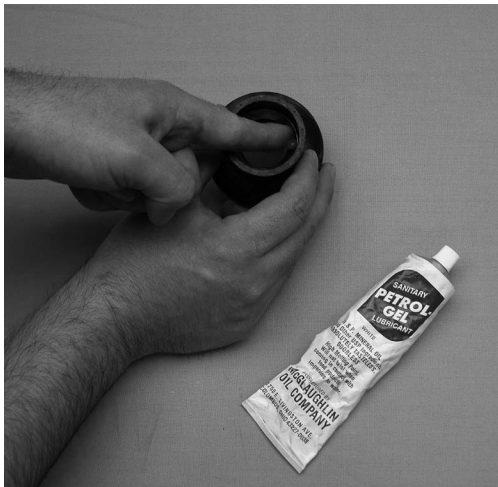
Figure 3-6 Lubricate Rear Seal
