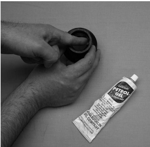
Figure 3-6 Lubricate Rear Seal
