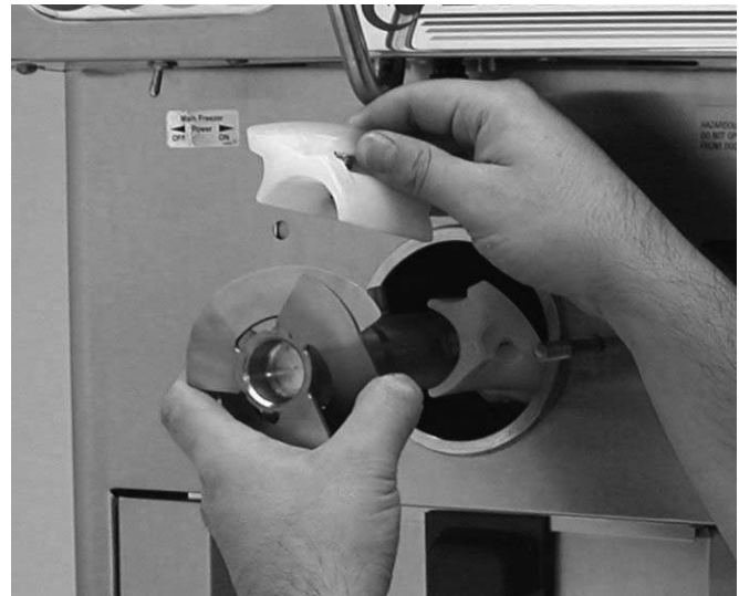
Figure 3-8 Removing Auger Shaft and Flights
