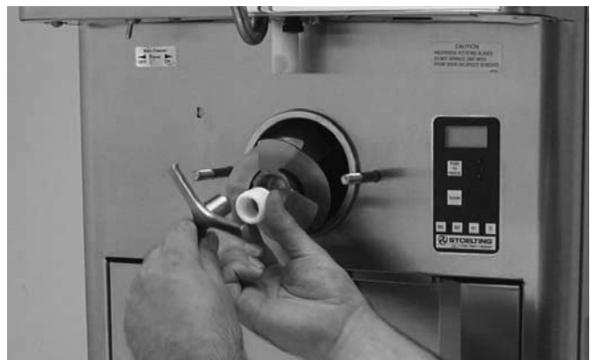
Figure 3-7 Removing Auger Support
